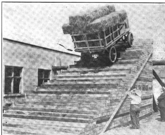
Jeffery Quad climbing 49 per cent. grade in factory test
